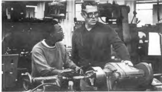
Byron Dorsey of Newark receives instructions from George Echols while performing a turning and shouldering operation.
